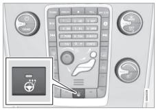
Button for steering wheel heating
