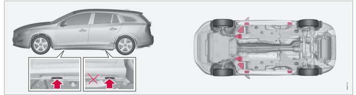
If a garage jack is used to lift the vehicle, it should be placed:
