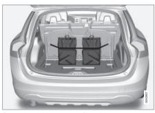
Grocery bag holder under the floor of the cargo area The grocery bag holder holds shopping bags in place.
