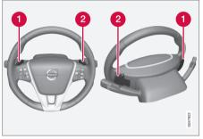
Steering-wheel mounted gear shift paddles
