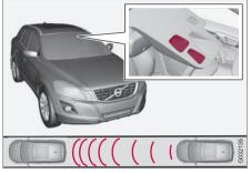
Location of the laser sensor in the windshield<sup>5</sup>
