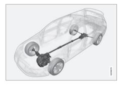
Under normal driving conditions, most of the engine's power is directed to the front wheels. However, if there is any tendency for the front wheels to spin, an electronically controlled coupling distributes power to the wheels that have the best traction.
