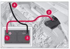
Connecting the jumper cables
