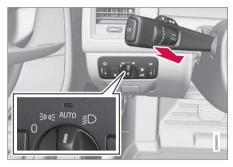
**Models with an analog instrument panel** When AHB is activated, the Symbol will illuminate in the instrument panel. The high beam indicator (SO) in the instrument panel will also illuminate when the high beams are on.
