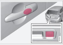
Models with keyless drive have a pressure-sensitive area on the outside door handles and a rubber-covered button next to the tailgate opening control
