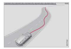
A camera monitors the painted lines marking the lane in which the vehicle is traveling and compares the direction of the road with the driver's movements of the steering wheel. The driver is alerted if the vehicle does not follow the lane smoothly.
