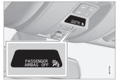
Occupant Weight Sensor (OWS) indicator light
