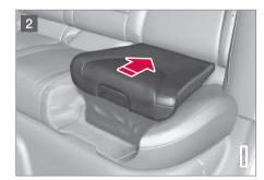
With the booster cushion in the stage 1 position, press the button (see the arrow in illustration 1).
