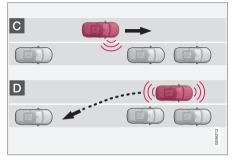
When the vehicle is backing up,  $\ensuremath{\mathsf{PAP}}$  will steer it into the parking space.
