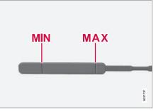
The oil level must be between the  $\ensuremath{\text{MIN}}$  and  $\ensuremath{\text{MAX}}$  marks on the dipstick
