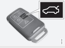
Tailgate unlock button on the remote key
