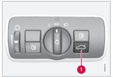
Press the button on the lighting panel (1) to unlock (but not open) the tailgate.
