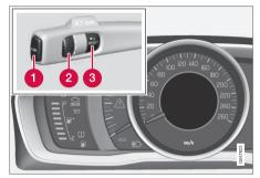
Analog Instrument panel and menu controls
