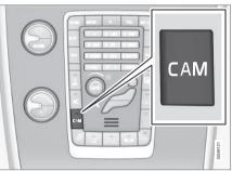
PAC is activated when the gear selector is moved to **R** if the system is selected in the **MY CAR** menu system or by pressing the **CAM** button in the center console. See My Car – introduction (p. 79) for a description of the menu system.
