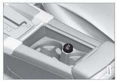
12-volt socket in the front tunnel console
