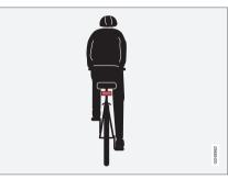
Optimal example of what the system considers to be a cyclist: clear body/bike contours, straight from behind and directly in front of the vehicle
