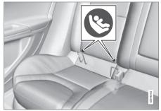
Symbols on the seat back upholstery mark the ISOFIX/LATCH anchor positions as shown. To access the anchors, kneel on the seat cushion and locate the anchors by feel. Always follow your child seat manufacturer's installation instructions, and use both ISOFIX/LATCH lower anchors and top tethers (p. 59) whenever possible.
