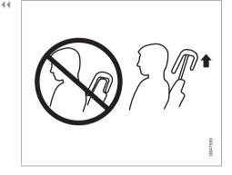
The center head restraint should be adjusted according to the passenger's height. The restraint should be carefully adjusted to support the occupant's head.
