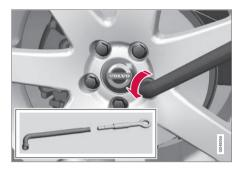
With the vehicle still on the ground, remove the plastic covers on the wheel nuts with the tool provided and use the lug wrench/towing eyelet to loosen the wheel nuts 1/2 – 1 turn by exerting downward (counterclockwise) pressure.
