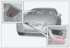
Camera and radar sensor<sup>6</sup>.
