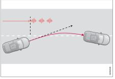
LKA provides vibrations in the steering wheel and steering assistance<sup>11</sup>.
