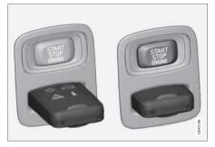
2. To turn off the alarm, insert the remote key into the ignition slot (also on vehicles with the optional keyless drive).
