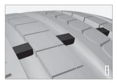
The letters **TWI** are printed on the side of the tire. When approximately 1/16" (1.6 mm) is left on the tread, these strips become visible and indicate that the tire should be replaced. Tires with less than 1/16" (1.6 mm) tread offer very poor traction.
